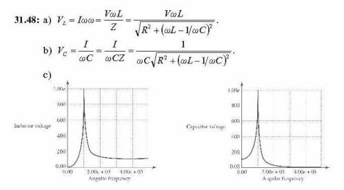
d) When the angular frequency is zero, the inductor has zero voltage while the capacitor has voltage of 100 V (equal to the total source voltage). At very high frequencies, the capacitor voltage goes to zero, while the inductor's voltage goes to 100 V  $t_{\rm c}$
